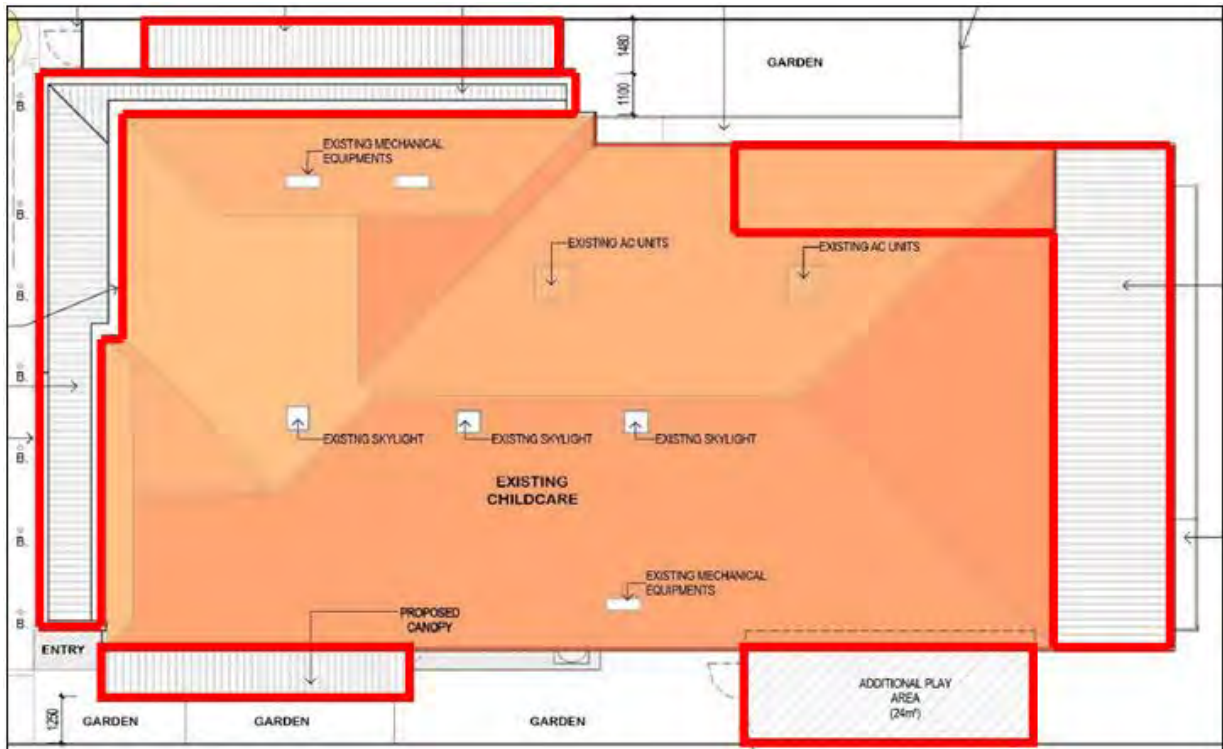
Figure 1: Proposed Building Works. Existing building shaded orange with proposed additions outlined in red.
