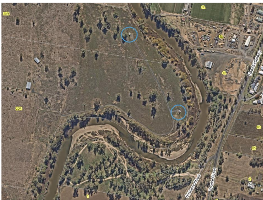
Figure 4 Location of bores in the northern portion of Council owned land on Bunglegumbie Rd - North-West Urban Release Area. These bores have associated electrical and pipeline infrastructure on the floodplain.
