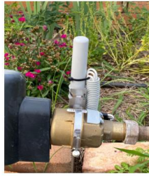
Clip on device - These attach to existing meters which are working fine and are not due for replacement in the coming years
