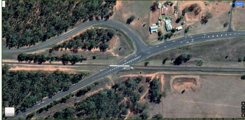
Figure 5. Google aerial photograph of the intersection, Boothenna Rd terminating at the Golden Hwy. Note the approach angle, level crossing and the auxiliary lanes provided on the Golden Hwy.
