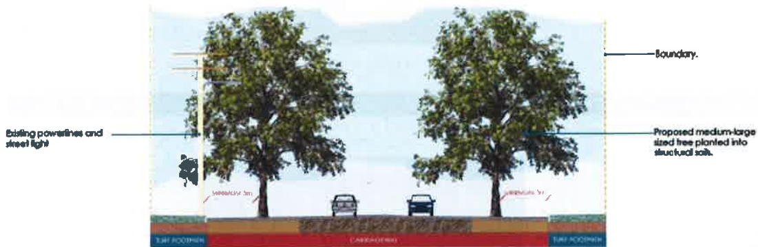
RESIDENTIAL ROAD LOCATION TYPE B | SECTION
