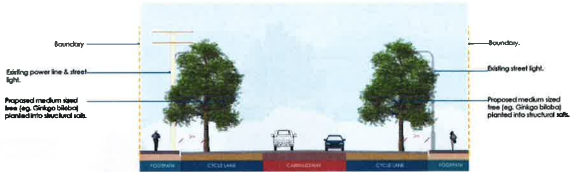
SUB-ARTERIAL LOCATION TYPE 4 | SECTION
