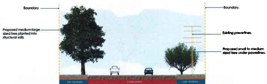
COLLECTOR ROAD LOCATION TYPE 6 | SECTION
