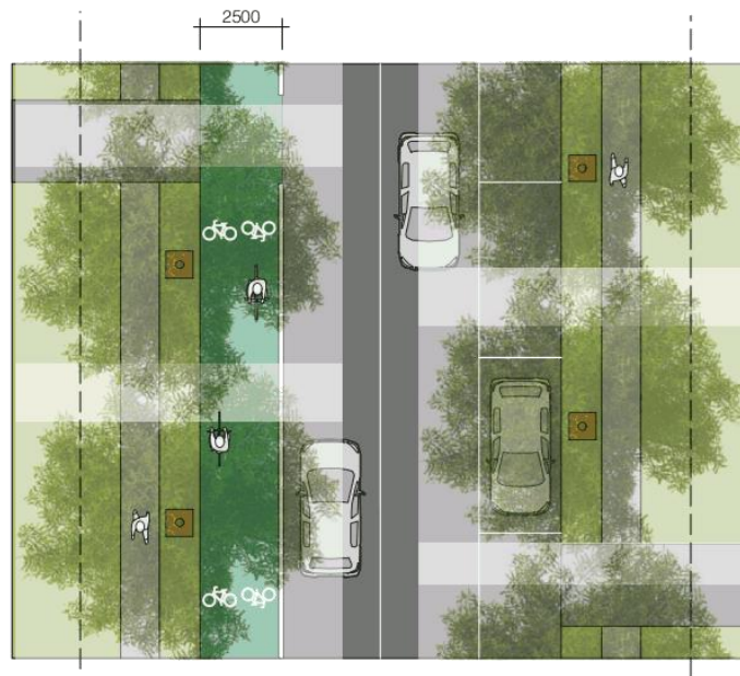
TYPE A: DEDICATED CYCLEWAY (ON ROAD) 1:250 A DEDICATED CYCLE LANE ON ONE SIDE OF CARRIAGE WAY AT ROAD LEVEL
