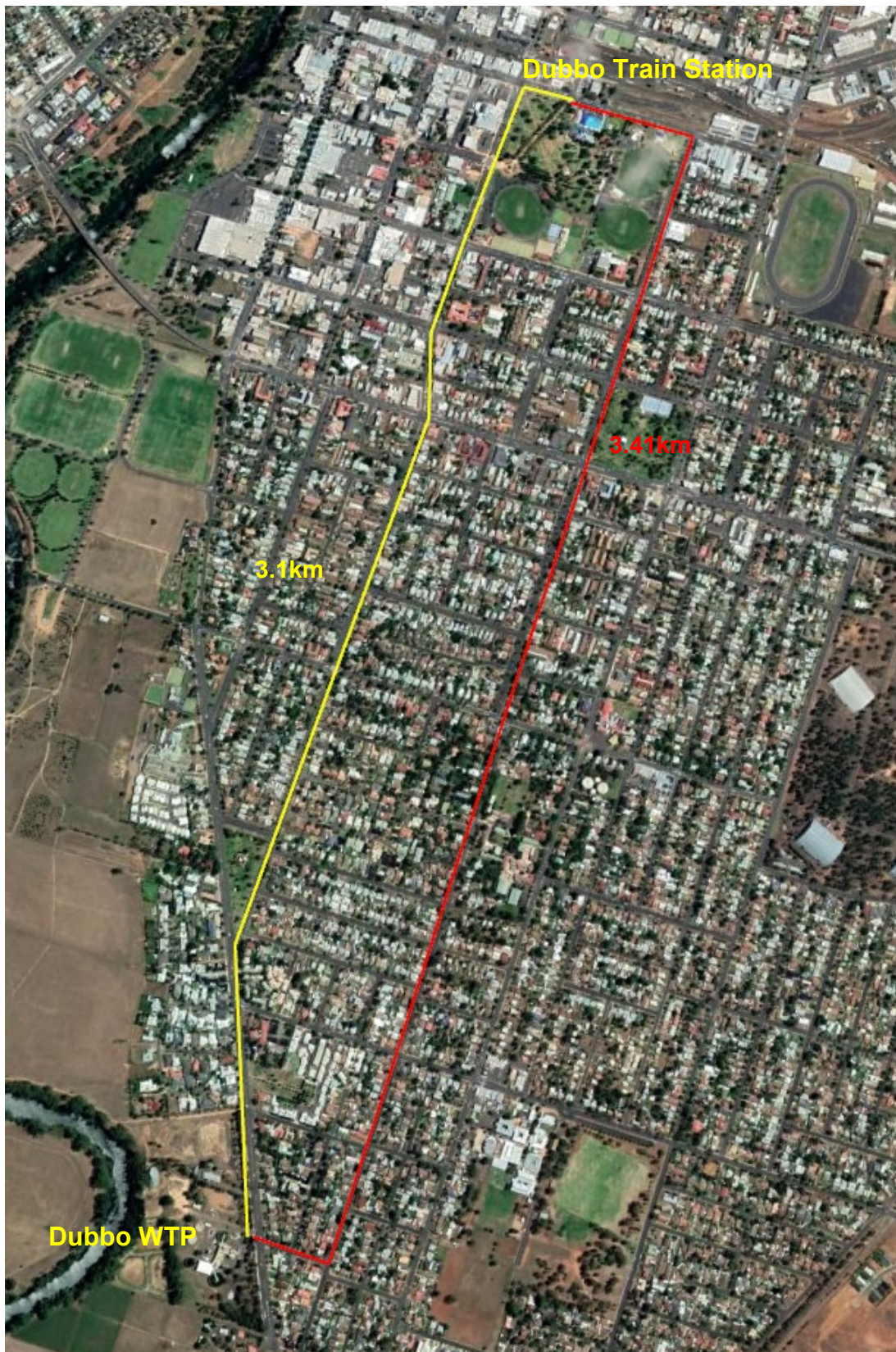
Appendix Figure C-2: Proposed 600mm Diameter 3.5km pipeline from train station to Dubbo WTP
