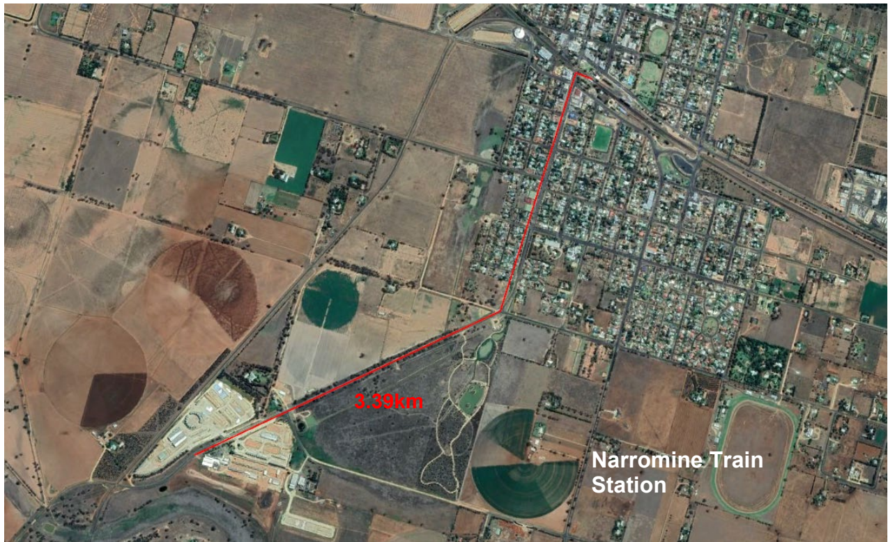
Appendix Figure C-1: Proposed 600mm Diameter 3.5 km pipeline from bore field to train station at Narromine
