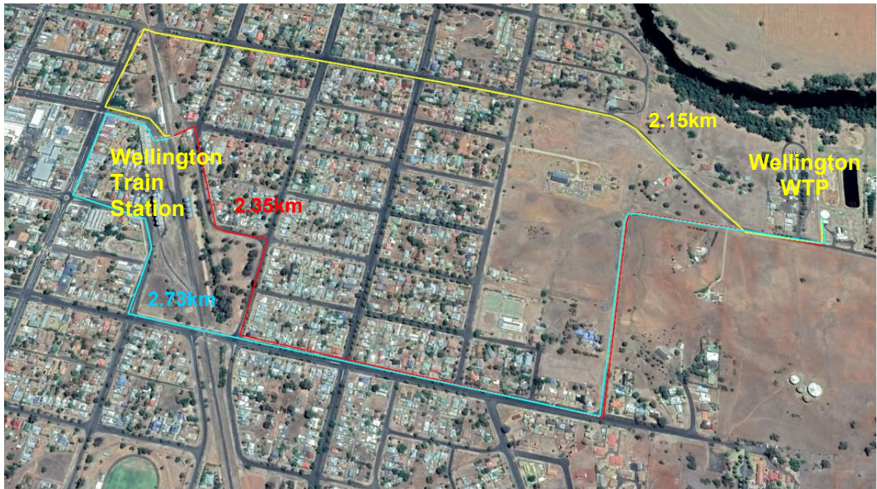
Appendix Figure C-3: Proposed 450mm Diameter 2.5km pipeline from train station to Wellington WTP
